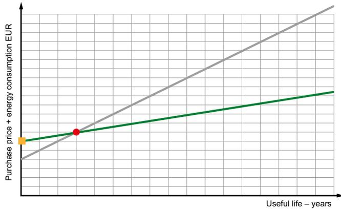
This general illustration is based on calculations of the transformer's energy consumption while energy costs remained constant at 13.4 ct/kWh (source: first energy) for 16 years. The wide variety of bandwidths result from the different transformer capacities.
